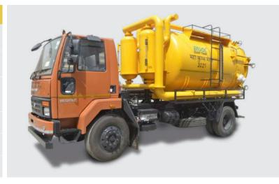
Note: Equipment Tank Volume, Capacity of Vacuum Pump and High Pressure jetting pump etc. can be changed and offered as per clients requirement.
